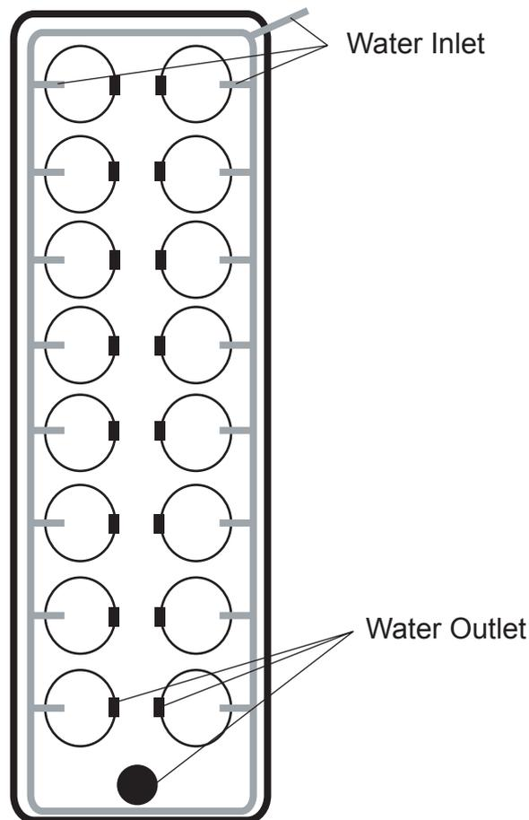
**Figure 11.** Diagram of flow through system showing 16 petri dishes, water inlet and outlet.
